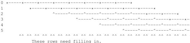
In this case, the first J - (J/G) = 9 - (9/3) = 6 jets of pass p + (6/3) = p + 2 collide with the last 6 jets of pass p. Only one row in every G = 2 rows is printed by this weave.
